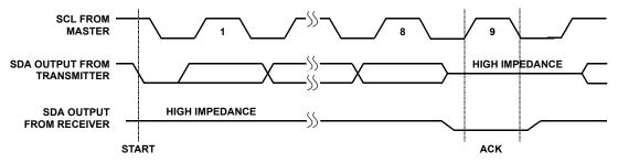
FIGURE 6. ACKNOWLEDGE RESPONSE FROM RECEIVER
