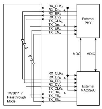
FIGURE 4. RMII PASSTHROUGH MODE
