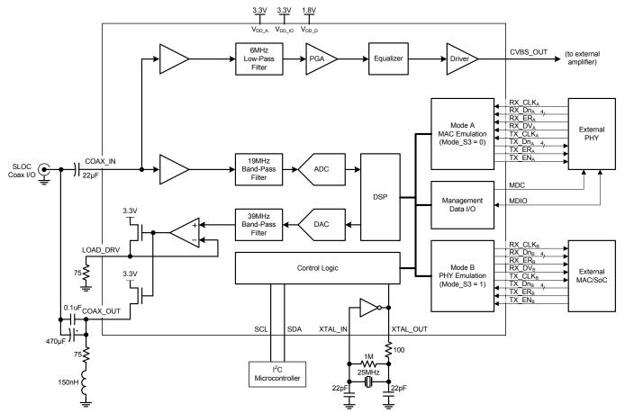
FIGURE 1. TW3811 INTERNAL BLOCK DIAGRAM
