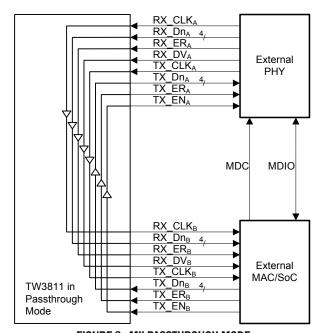
FIGURE 3. MII PASSTHROUGH MODE
