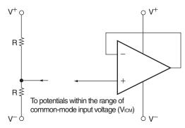
**Remark** A midpoint potential of V<sup>+</sup> and V<sup>-</sup> is applied to this example.
