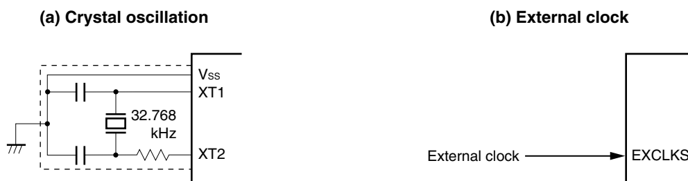
Figure 6-10. Example of External Circuit of XT1 Oscillator
