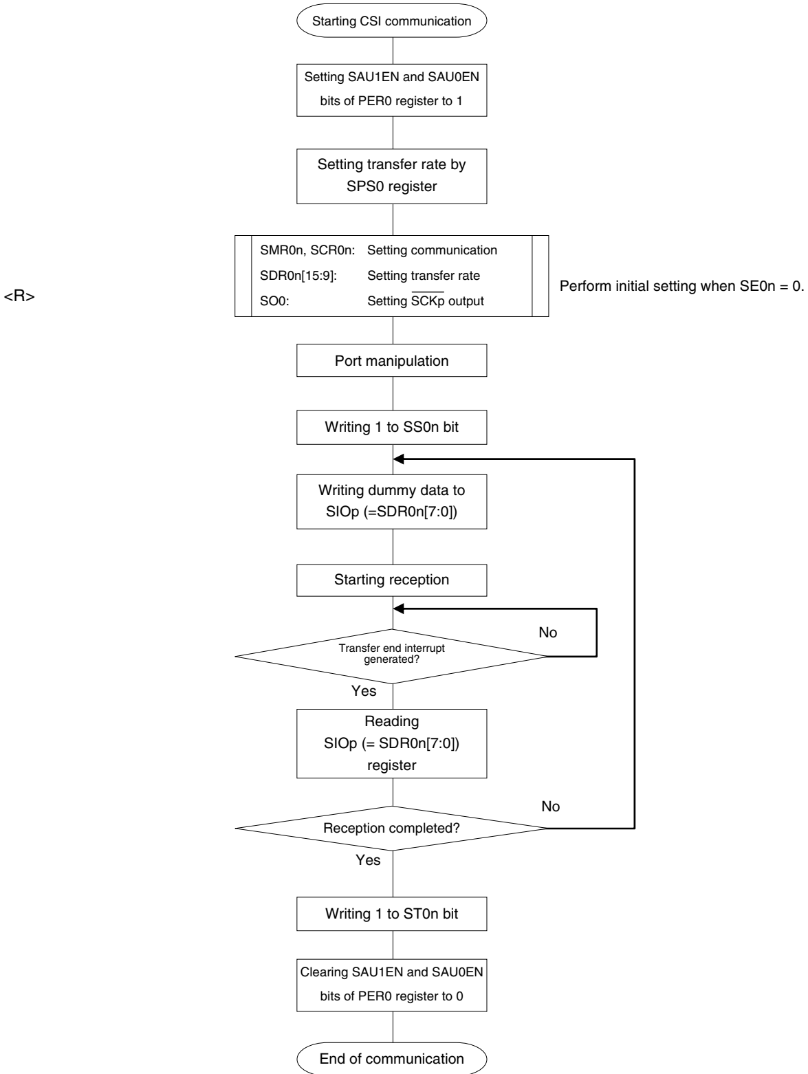
Figure 11-37. Flowchart of Master Reception (in Single-Reception Mode)
