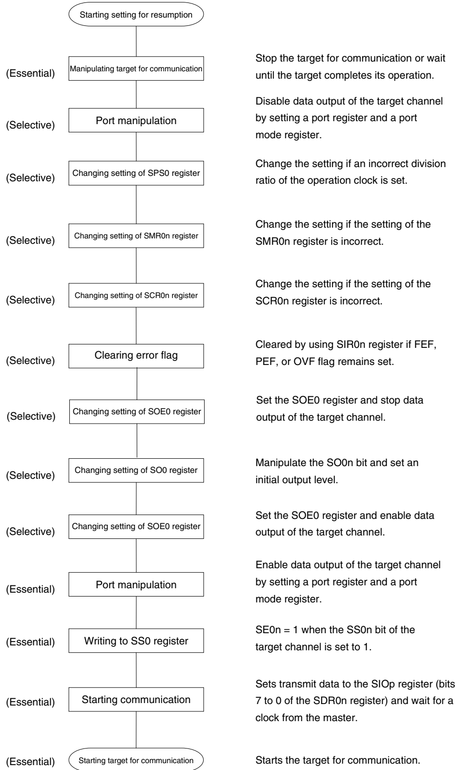
Figure 11-51. Procedure for Resuming Slave Transmission
