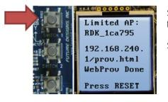
**STEP 4**: Perform the <u>provisioning</u> sequence (steps 1-5 on page 4). You should see the following message displayed on the LCD screen.
