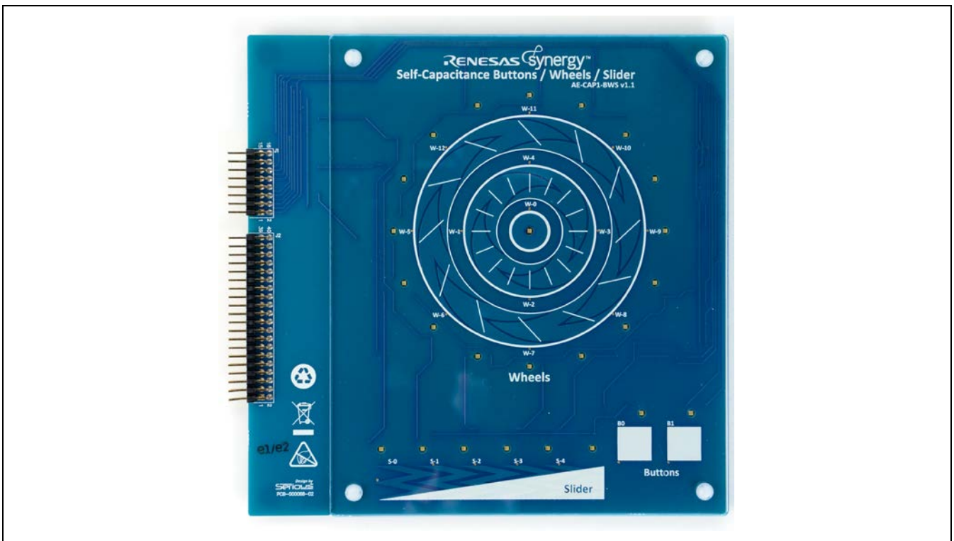
Figure 3 AE-CAP1-BWS Application Board
