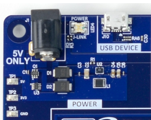
Figure 4: Power Section of Main Board
