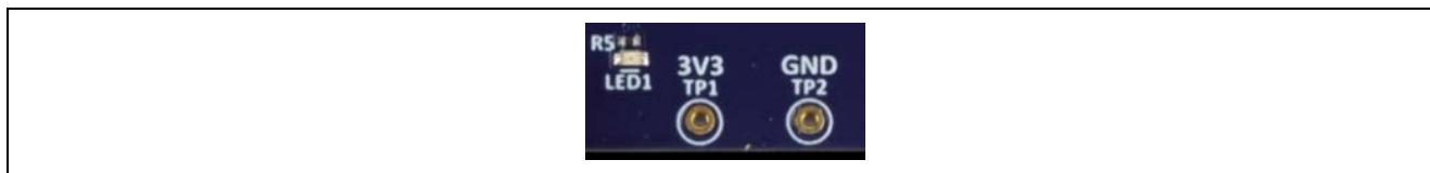
Figure 7. TP1, TP2, and LED1 on Target Board
