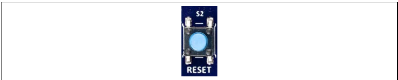
Figure 18. Reset Switch (S2) on Target Board
