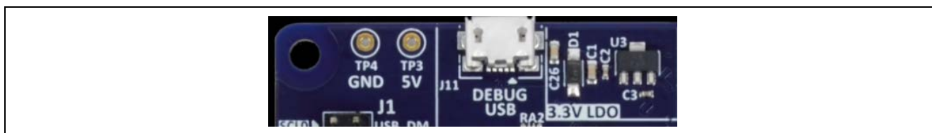
Figure 6. USB Debug Connector (J11), TP3, and TP4 on Target Board
