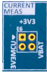
Figure 12. E6 on Target Board (Top Side)
