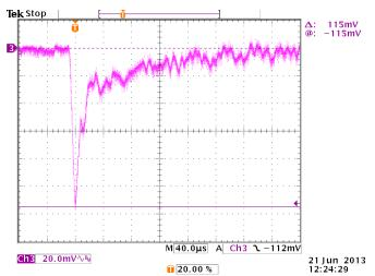
FIGURE 10. (3 - 5 A LOAD STEP,  $di/dt = 2.5A/\mu s$
