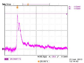
FIGURE 11. (5 - 3 A LOAD STEP,  $di/dt = 2.5A/\mu s$
