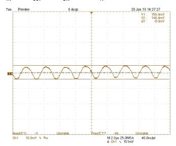
FIGURE 9. OUTPUT RIPPLE MEASURED ACROSS C3
