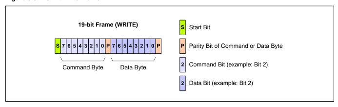
The incoming serial signal will be sampled at a 512 kHz clock rate. This protocol is very tolerant to clock skew and can easily tolerate baud rates in the 6 kHz to 48 kHz range.
