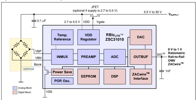
Figure 2.1 ZSC31010 Block Diagram
