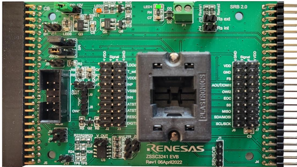
Figure 6. Evaluation Board LED Status after Starting GUI
