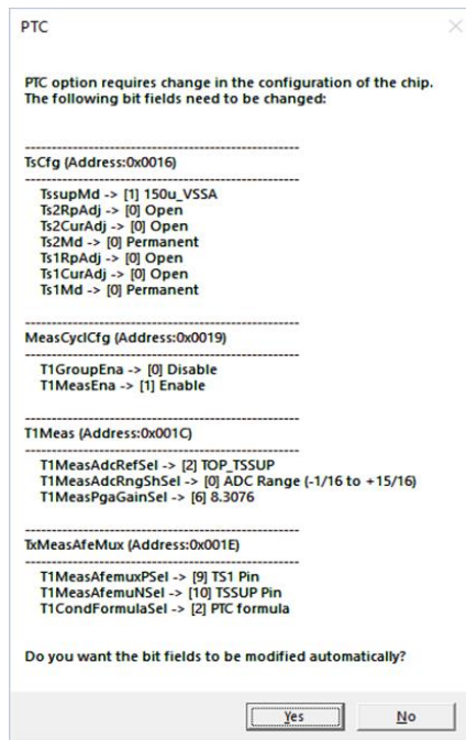
Figure 24. IC Settings for PT1000 Setup (Configure Pin TS1 and TS2, Measurement Uses Pin TS1)
