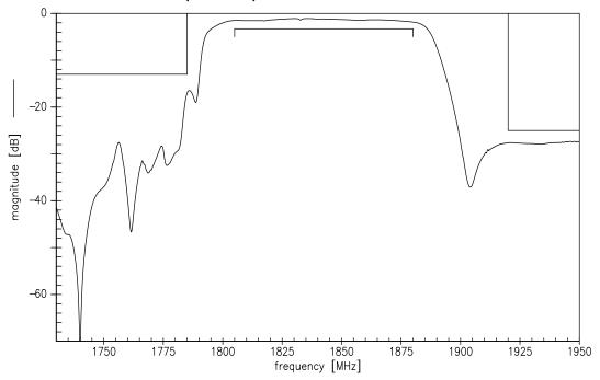
Transfer function of Filter 1 (GSM1800) - Wideband
