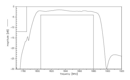
Transfer function of Filter 2 (GSM1800) - Wideband
