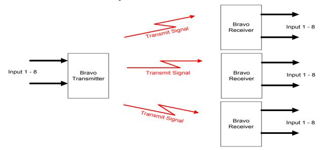
In this application the outputs at each of the receivers will track the inputs at the transmitter.
