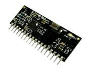
**BRAVO-T868** - 868 MHz SMART Radio Module with 8 digital outputs.
