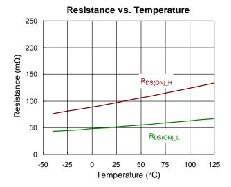
Figure 13. RT6253A/B RDS(ON) vs. Temperature
