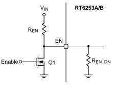
Figure 8. Digital Enable Control Circuit
