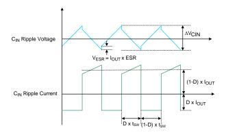
Figure 1. CIN Ripple Voltage and Ripple Current
