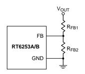
Figure 2. Output Voltage Setting
