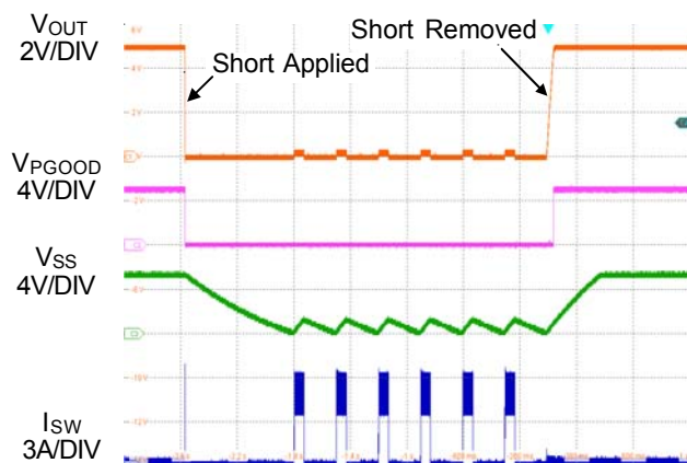
Figure 3. Short Circuit Protection and Recovery
