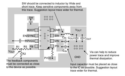
Figure 3. PCB Layout Guide
