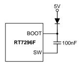
Figure 2. External Bootstrap Diode
