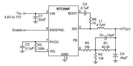
Note: All input and output capacitance in the suggested parameter mean the effective capacitance. The effective capacitance needs to consider any De-rating Effect like DC Bias.
