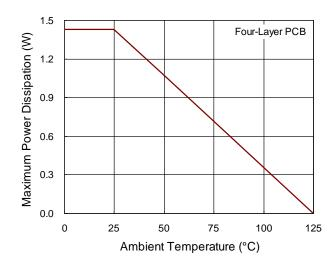
Figure 3. Derating Curve of Maximum Power
