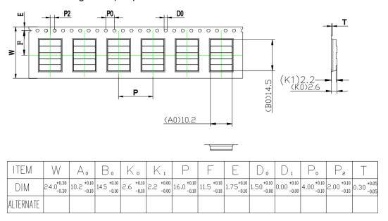
Figure 14: BMD-330-A-R-00 carrier tape dimensions
