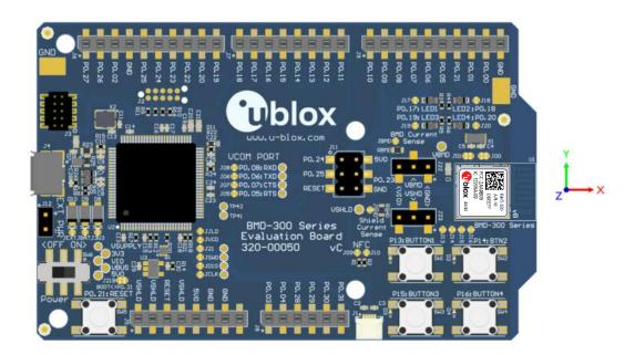
Figure 9: BMD-330 Evaluation kit X-Y-Z orientation
