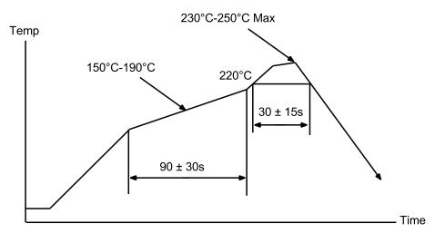
Figure 16: Reflow Profile for Lead Free Solder
