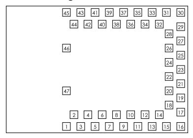
Figure 2: BMD-330 Pin assignment
