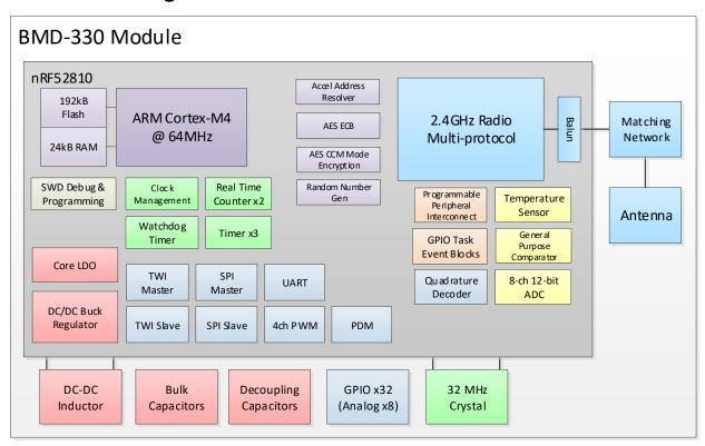
Figure 1: Block diagram of BMD-330
