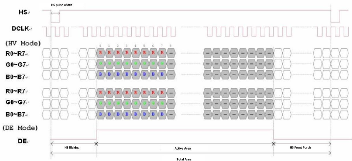
Figure 12. Horizontal input timing diagram
