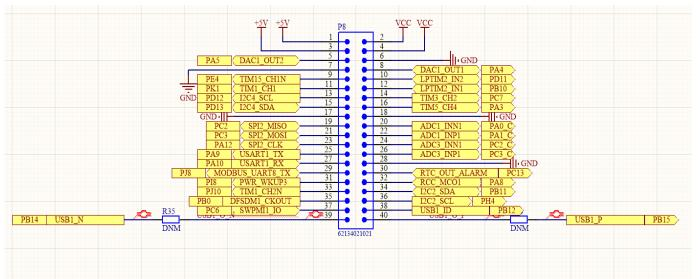
Each of the GPIO pins can be configured by software as output (push-pull or open-drain, with or without pull-up or pull-down), as input (floating, with or without pull-up or pull-down) or as peripheral alternate function. Most of the GPIO pins are shared with digital or analog alternate functions. Please refer to the datasheet of MCU STM32H747XIH6 for more details.
