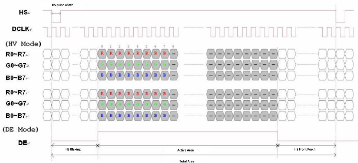
Figure 12. Horizontal input timing diagram
