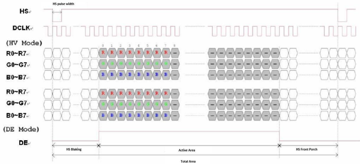
Figure 5. Horizontal input timing diagram
