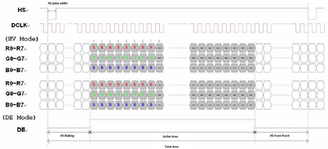
Figure 5. Horizontal input timing diagram
