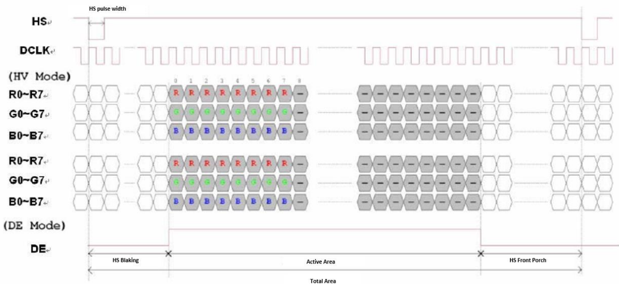
Figure 12. Horizontal input timing diagram
