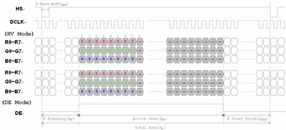
Figure 7. Horizontal input timing diagram
