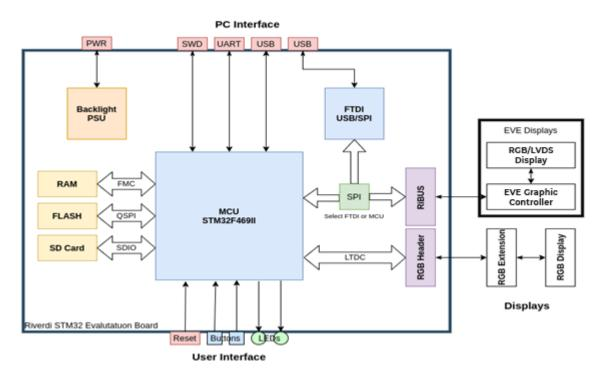
The Riverdi STM32 Evaluation board contains all necessary components for successful development of graphic applications, including:
