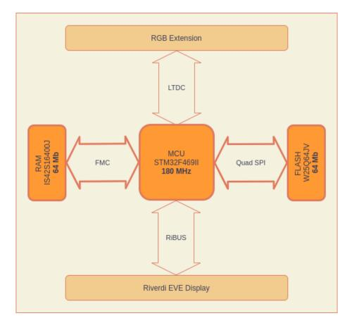
The key component, the STM32F469II Cortex M4 microcontroller, is running with clock frequency up to 180MHz and carry 2MB of the non-volatile and 384KB of internal RAM. Alongside the microcontroller, the evaluation board contains additional IS42S16400J 64Mb external RAM connected through 32-bit data bus and W25Q64JV 64Mb external Flash memory, connected through Quad SPI interface.
