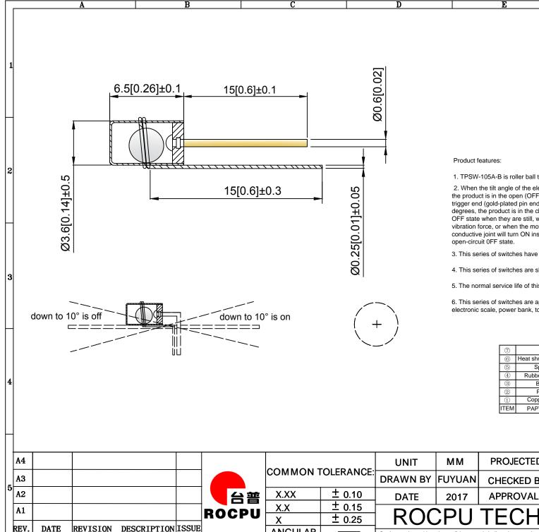
**ROCPU Product features** Voltage: < 12V Current: < 20mA Conduction time: 2ms Closed circuit resistance: < 1 ohm Open circuit resistance: > 1 ohm High temperature resistance: 120 degrees Terminal tension: 500gf / min Humidity: 25~95%RH Operating life: 100000 times
