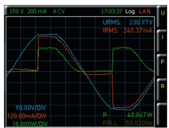
Waveform function: load with phase-angle control.
