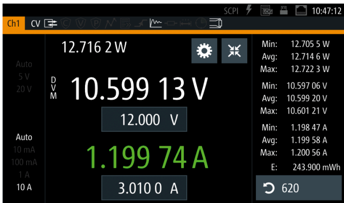
The internal digital voltmeter of the R&S®NGM200 power supplies can optionally be used to measure at any point in the customer's circuitry.
