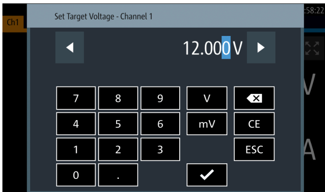
Numerical values can be entered using the virtual touchscreen keyboard or the rotary knob.
