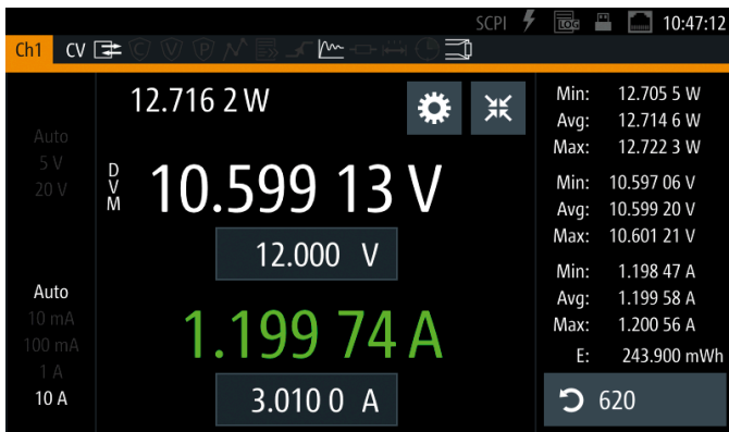
The internal digital voltmeter of the R&S®NGM200 power supplies can optionally be used to measure at any point in the customer's circuitry.
