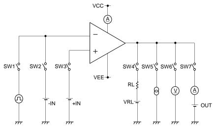
Figure 50. Test Circuit 2 (one channel only)
