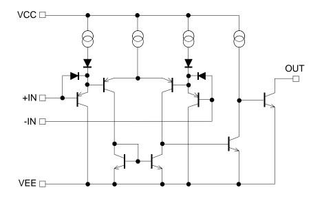
Figure 1. Simplified schematic (one channel only)
