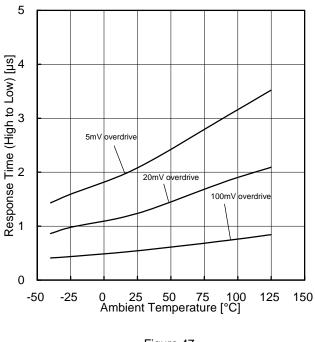
Figure 47. Response Time (High to Low) vs Ambient Temperature (VCC=5V, V<sub>RL</sub>=5V, R<sub>L</sub>=5.1kΩ)
