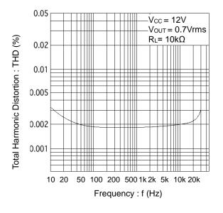
Figure 9. Total Harmonic Distortion vs Frequency
