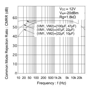
Figure 10. Common Mode Rejection Ratio vs Frequency
