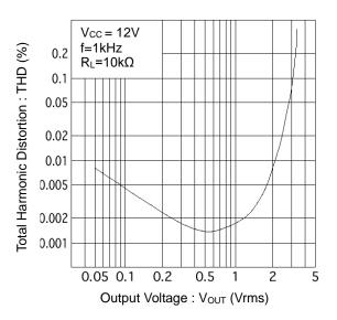
Figure 8. Total Harmonic Distortion vs Output Voltage
