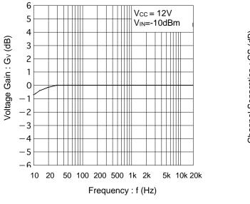
Figure 5. Voltage Gain vs Frequency
