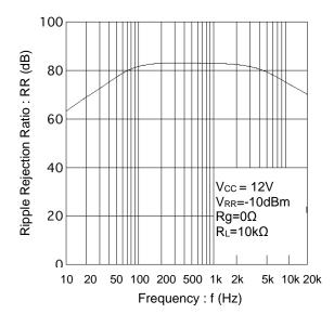
Figure 7. Ripple Rejection Ratio vs Frequency
