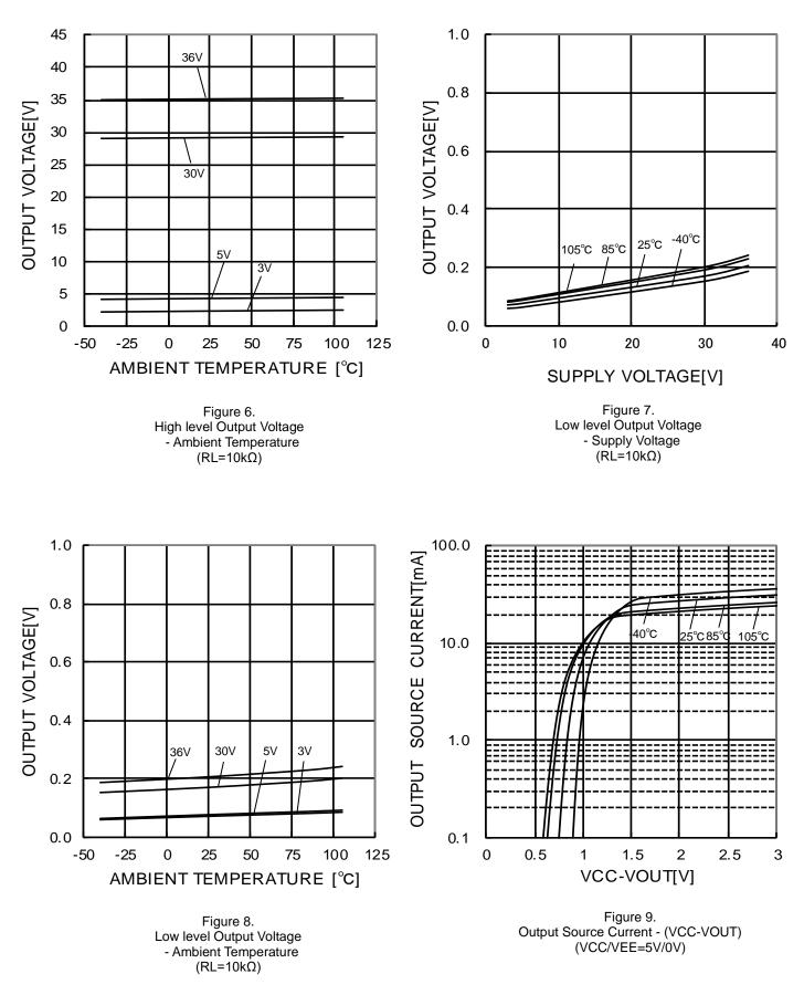
(\*) The above data is measurement value or typical sample, it is not guaranteed. BA3472 : -40°C~+85°C BA3472R : -40°C~+105°C
