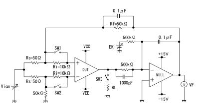
Figure 48. Test circuit 1 (one channel only)
