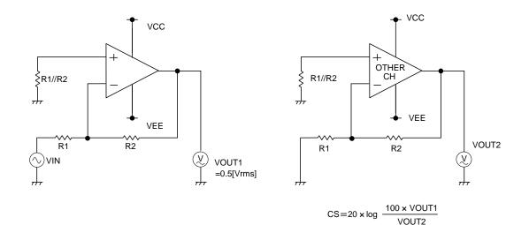
Figure 51. Test circuit 3 (Channel Separation)
