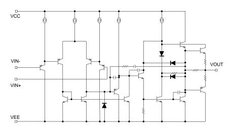
Figure 1. Simplified schematic (one channel only)
