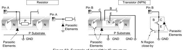
Figure 53. Example of monolithic IC structure
