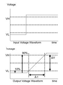
Figure 50. Slew rate input output wave
