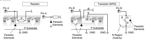
Figure 16. Example of Monolithic IC Structure
