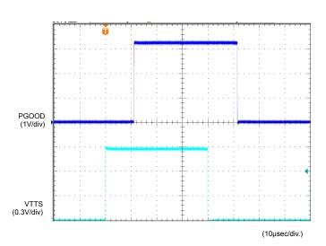
Figure 15. PGOOD Delay (TSD OFF-TSD ON)
