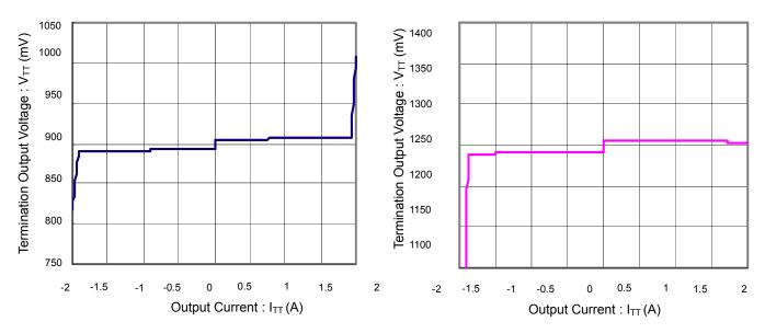
Figure 1. Termination Output Voltage vs Output Current (DDR2)
