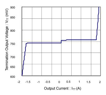
Figure 3. Termination Output Voltage vs Output Current (DDR3)
