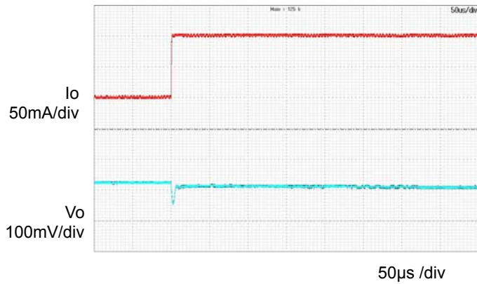
Figure 12. Transient Response ( T_a=105^\circ\text{C} ) ( I_o = 0\text{A} \rightarrow 0.1\text{A} )
