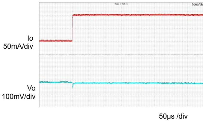
Figure 10. Transient Response ( T_a=-40^\circ\text{C} ) ( I_o = 0\text{A} \rightarrow 0.1\text{A} )
