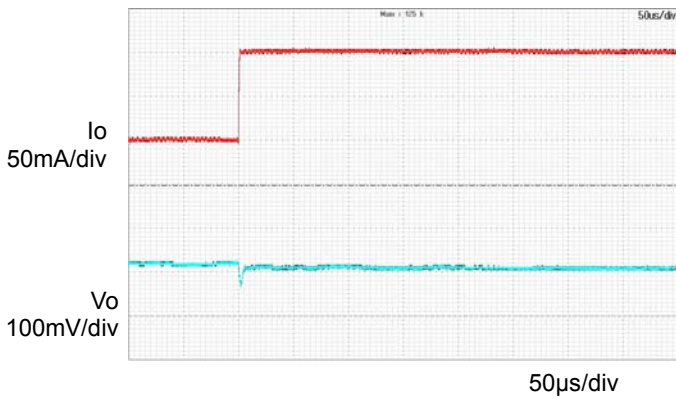
Figure 8. Transient Response ( T_a=25^\circ\text{C} ) ( I_o = 0\text{A}\rightarrow 0.1\text{A} )
