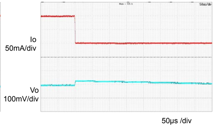
Figure 11. Transient Response ( T_a=-40^\circ\text{C} ) ( I_o = 0.1\text{A} \rightarrow 0\text{A} )
