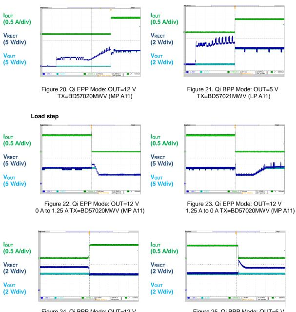
Figure 24. Qi BPP Mode: OUT=12 V 0 A to 1.0 A TX=BD57021MWV (LP A11) Figure 25. Qi BPP Mode: OUT=5 V 1.0 A to 0 A TX=BD57021MWV (LP A11)
