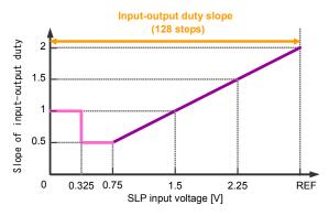
Figure 24. Relations of SLP terminal voltage and the input-output duty slope characteristics
