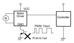
Figure 45. GND Line PWM Switching Prohibited
