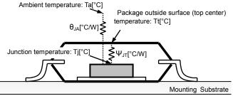
Figure 47. Thermal Resistance Model of Surface Mount
