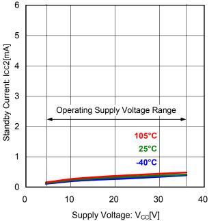
Figure 2. Standby Current vs Supply Voltage
