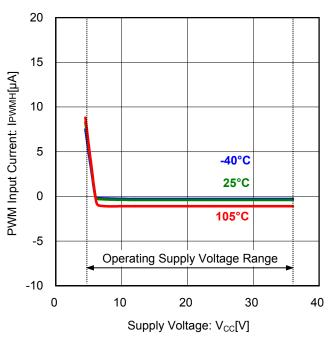
Figure 4. PWM Input Current vs Supply Voltage (V<sub>PWM</sub>=5V)
