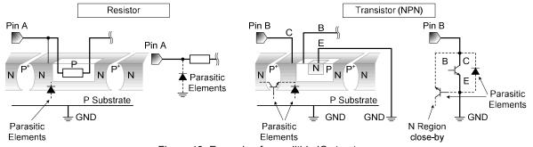
Figure 49. Example of monolithic IC structure
