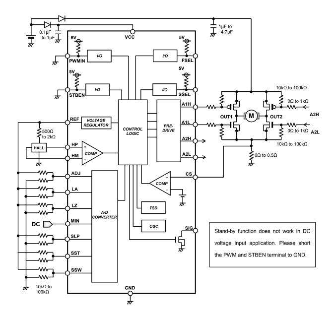
When a function is not used, do not let the A/D converter input terminal open.
