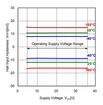
Figure 3. Hall Input Hysteresis vs Supply Voltage
