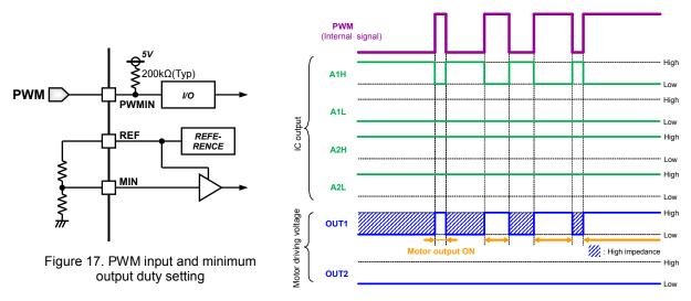
Figure 18. Output PWM operation timing chart
