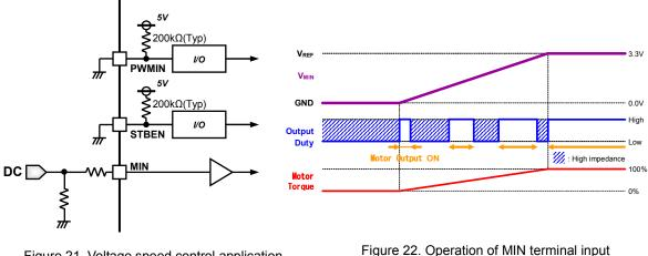
Figure 21. Voltage speed control application
