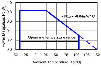
Figure 48. Power Dissipation vs Ambient Temperature
