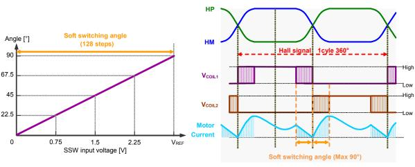
Figure 28. Relations of SSW terminal voltage and the angle of soft switching
