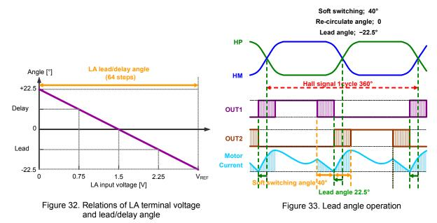
LA setting decide the point of output changing timing, PWM soft switching and LZ re-circulate angle are decided based on that point. When PWM soft switching, re-circulate, lead angle setting are changed each, operational example image is show in Figure 34.
