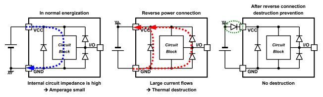
Figure 44. Flow of Current When Power is Connected Reversely
