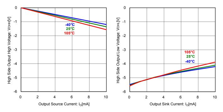
Figure 9. High Side Output High Voltage vs Source Current ( $V_{CC}$ =12V, differential voltage to Vcc)
