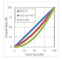
Figure 27. Input duty vs output duty characteristics
