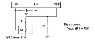
Figure 43. Application near of Hall Signal
