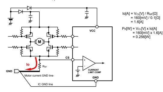
Figure 40. Current limit setting and GND line
