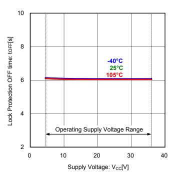
Figure 16. Lock Protection OFF Time vs Supply Voltage
