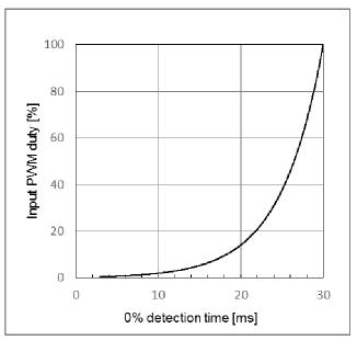
Figure 39. Input PWM DUTY vs 0% detection time
