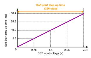
Figure 35. Relations of SST terminal voltage and soft start step up time
