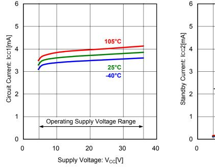
Figure 1. Circuit Current vs Supply Voltage
