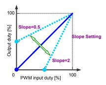
Figure 23. Properties of input-output duty slope setting
