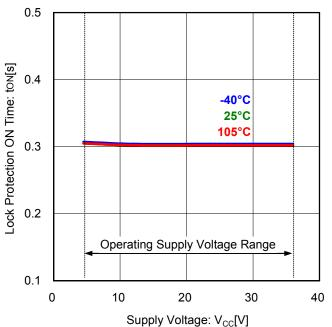
Figure 15. Lock Protection ON Time vs Supply Voltage
