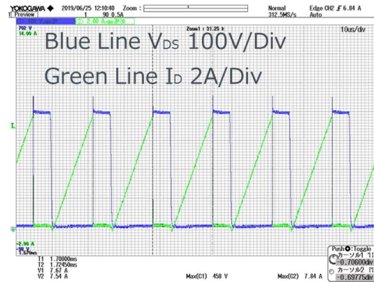
Figure 19. V_{DS}, I_D ZOOM
