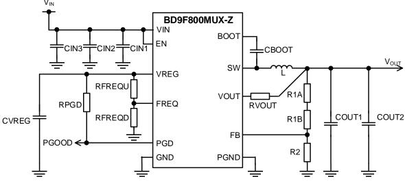
Figure 81. Application Circuit
