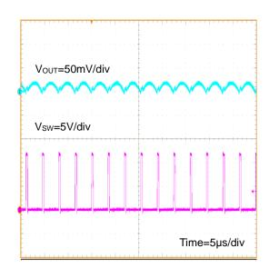
Figure 55. Vout Ripple Iout=8A (VIN=12V, VOUT=1V, FREQ=L(300kHz))
