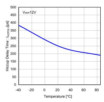
Figure 27. Hiccup Delay Time vs Temperature
