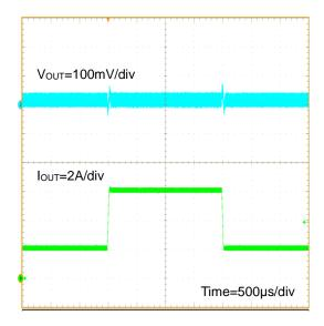
Figure 69. Load Transient Response I<sub>OUT</sub>=2A - 6A (V<sub>IN</sub>=12V, V<sub>OUT</sub>=1.2V, FREQ=H(600kHz))
