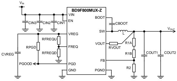
Figure 56. Application Circuit
