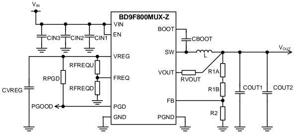
Figure 71. Application Circuit
