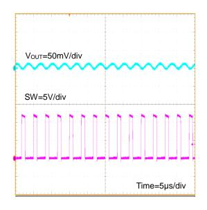
Figure 75.  $V_{OUT}$  Ripple  $I_{OUT}$ =8A ( $V_{IN}$ =12V,  $V_{OUT}$ =3.3V, FREQ=L(300kHz))
