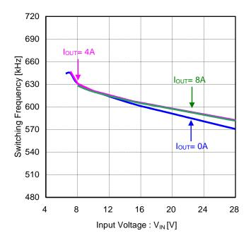
Figure 45. Switching Frequency vs Input Voltage (Vout=5V, FREQ=H(600kHz))
