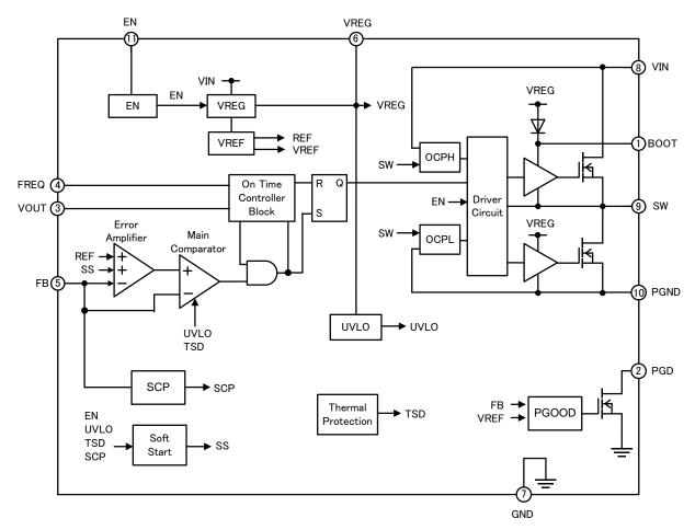
Figure 3. Block Diagram
