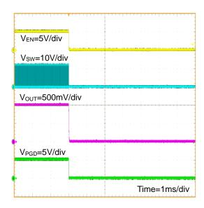
Figure 35. Shutdown Waveform (V<sub>EN</sub>=5V to 0V) (V<sub>IN</sub>=12V, V<sub>OUT</sub>=1V, FREQ=L(300kHz), R<sub>LOAD</sub>=0.125 $\Omega$ )
