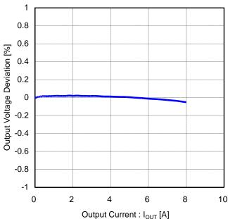
Figure 36. Load Regulation (V<sub>IN</sub>=12V, V<sub>OUT</sub>=1V, FREQ=L(300kHz))
