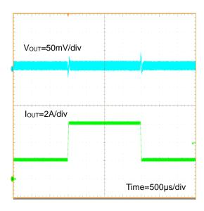
Figure 54. Load Transient Response I<sub>OUT</sub>=2A - 6A (V<sub>IN</sub>=12V, V<sub>OUT</sub>=1V, FREQ=L(300kHz))
