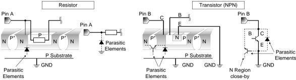
Figure 97. Example of monolithic IC structure
