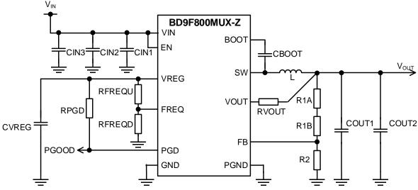
Figure 76. Application Circuit
