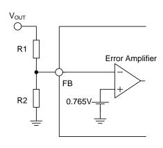
Figure 93. Feedback Resistor Circuit
