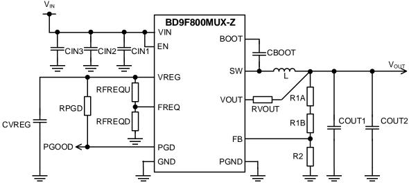
Figure 86. Application Circuit
