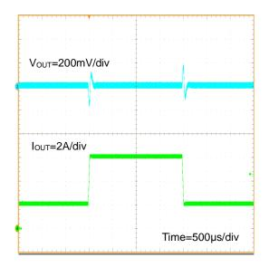
Figure 84. Load Transient Response I<sub>OUT</sub>=2A - 6A (V<sub>IN</sub>=12V, V<sub>OUT</sub>=5V, FREQ=L(300kHz))
