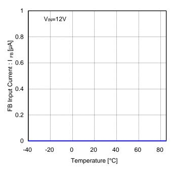
Figure 15. FB Input Current vs Temperature
