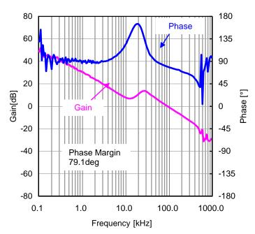
Figure 78. Loop Response  $I_{OUT}$ =8A ( $V_{IN}$ =12V,  $V_{OUT}$ =3.3V, FREQ=H(600kHz))
