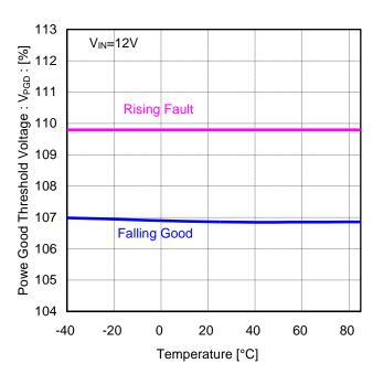
Figure 23. Power Good Threshold Voltage vs Temperature
