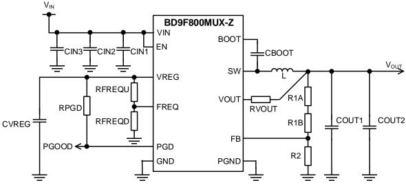
Figure 51. Application Circuit
