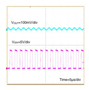
Figure 85. Vout Ripple Iout=8A ( $V_{IN}$ =12V,  $V_{OUT}$ =5V, FREQ=L(300kHz))
