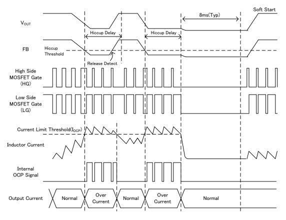
Figure 49. Over current protection timing chart
