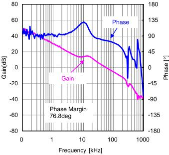
Figure 73. Loop Response  $I_{OUT}$ =8A ( $V_{IN}$ =12V,  $V_{OUT}$ =3.3V, FREQ=L(300kHz))
