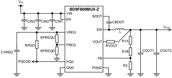
Figure 66. Application Circuit
