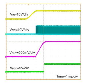
Figure 32. Start-up Waveform ( $V_{IN}=V_{EN}$ ) ( $V_{IN}=12V$ ,  $V_{OUT}=1V$ , FREQ=L(300kHz),  $R_{LOAD}=0.125\Omega$ )
