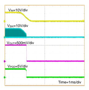
Figure 33. Shutdown Waveform  $(V_{IN}=V_{EN})$   $(V_{IN}=12V, V_{OUT}=1V, FREQ=L(300kHz), R_{LOAD}=0.125\Omega)$
