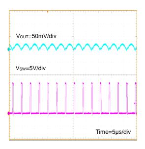
Figure 65. Vout Ripple Iout=8A (V<sub>IN</sub>=12V, V<sub>OUT</sub>=1.2V, FREQ=L(300kHz))
