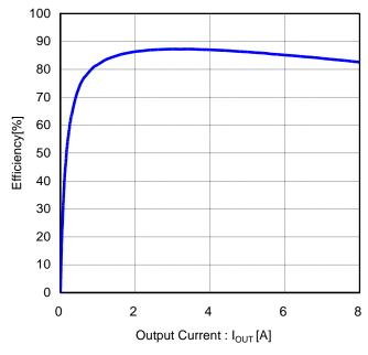
Figure 67. Efficiency vs Output Current (V<sub>IN</sub>=12V, V<sub>OUT</sub>=1.2V, FREQ=H(600kHz))
