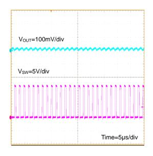
Figure 80.  $V_{OUT}$  Ripple  $I_{OUT}$ =8A ( $V_{IN}$ =12V,  $V_{OUT}$ =3.3V, FREQ=H(600kHz))
