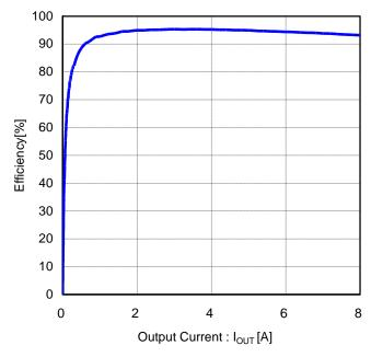
Figure 87. Efficiency vs Output Current  $(V_{IN}=12V, V_{OUT}=5V, FREQ=H(600kHz))$
