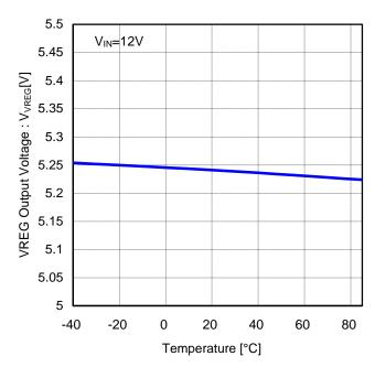
Figure 11. VREG Output Voltage vs Temperature
