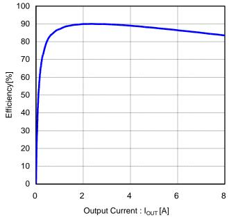
Figure 62. Efficiency vs Output Current (V<sub>IN</sub>=12V, V<sub>OUT</sub>=1.2V, FREQ=L(300kHz))
