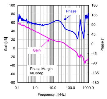
Figure 63. Loop Response I<sub>OUT</sub>=8A (V<sub>IN</sub>=12V, V<sub>OUT</sub>=1.2V, FREQ=L(300kHz))
