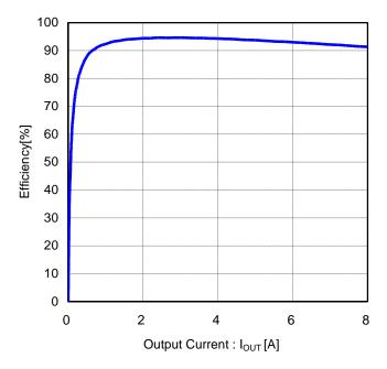
Figure 72. Efficiency vs Output Current (V<sub>IN</sub>=12V, V<sub>OUT</sub>=3.3V, FREQ=L(300kHz))
