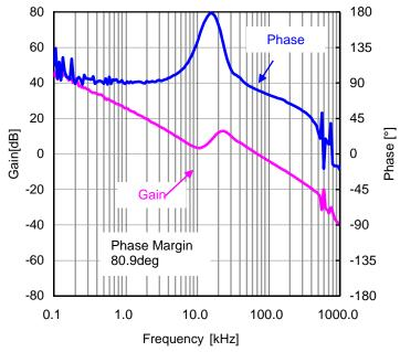
Figure 88. Loop Response I<sub>OUT</sub>=8A (V<sub>IN</sub>=12V, V<sub>OUT</sub>=5V, FREQ=H(600kHz))
