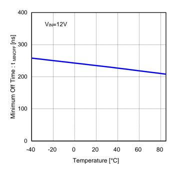
Figure 19. Minimum Off Time vs Temperature
