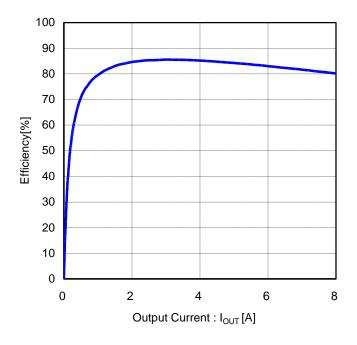
Figure 57. Efficiency vs Output Current  $(V_{IN}=12V, V_{OUT}=1V, FREQ=H(600kHz))$
