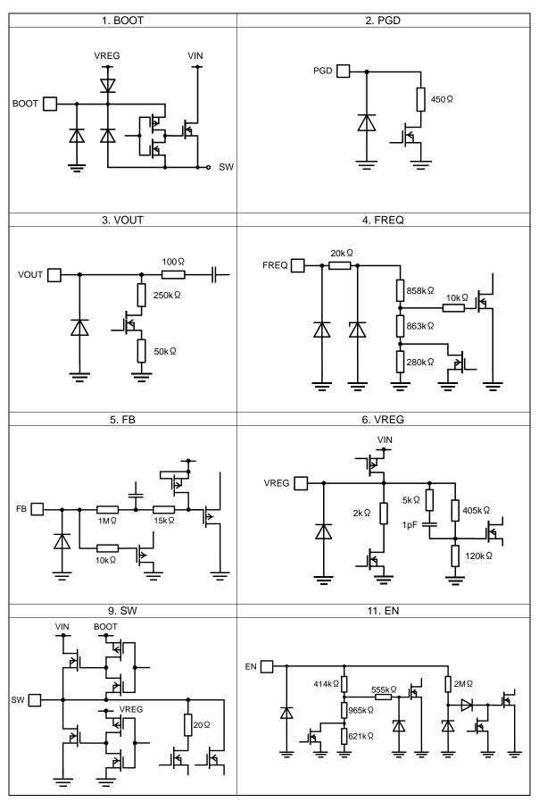
Figure 96. I/O equivalence circuit
