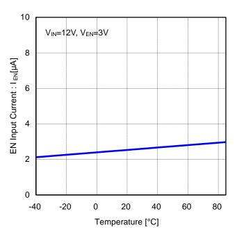
Figure 7. EN Input Current vs Temperature
