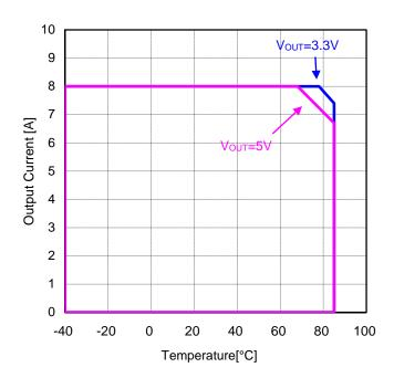
Figure 31. Operational Range V<sub>IN</sub>=24V, FREQ=H(600kHz), (Tj<150°C) (Measured on FR-4 board 85 mm x 85 mm, Copper Thickness: Top and Bottom 70μm, 2 Internal Layers 35μm)
