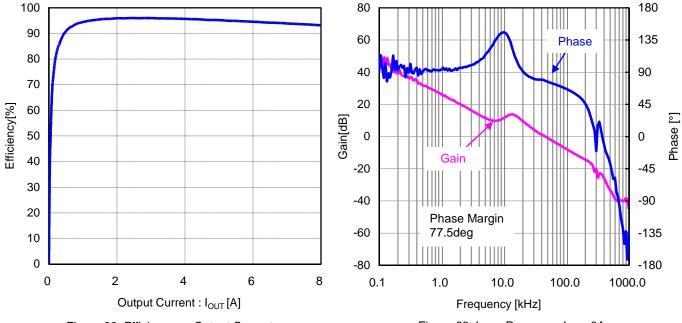
Figure 82. Efficiency vs Output Current ( $V_{IN}$ =12V,  $V_{OUT}$ =5V, FREQ=L(300kHz))
