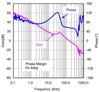
Figure 58. Loop Response  $I_{OUT}$ =8A ( $V_{IN}$ =12V,  $V_{OUT}$ =1V, FREQ=H(600kHz))
