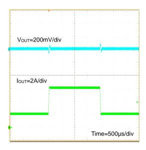
Figure 79. Load Transient Response I<sub>OUT</sub>=2A - 6A (V<sub>IN</sub>=12V, V<sub>OUT</sub>=3.3V, FREQ=H(600kHz))
