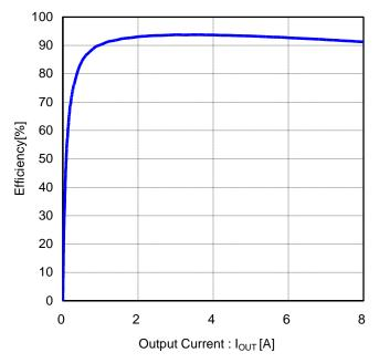
Figure 77. Efficiency vs Output Current (V<sub>IN</sub>=12V, V<sub>OUT</sub>=3.3V, FREQ=H(600kHz))
