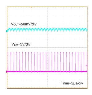
Figure 60. Vout Ripple Iout=8A (VIN=12V, VOUT=1V, FREQ=H(600kHz))
