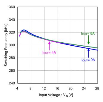
Figure 42. Switching Frequency vs Input Voltage (Vout=3.3V, FREQ=L(300kHz))
