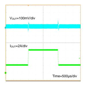
Figure 64. Load Transient Response I<sub>OUT</sub>=2A - 6A (V<sub>IN</sub>=12V, V<sub>OUT</sub>=1.2V, FREQ=L(300kHz))
