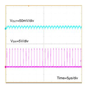
Figure 70. Vout Ripple Iout=8A (V<sub>IN</sub>=12V, V<sub>OUT</sub>=1.2V, FREQ=H(600kHz))
