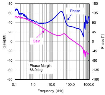
Figure 68. Loop Response I<sub>OUT</sub>=8A (V<sub>IN</sub>=12V, V<sub>OUT</sub>=1.2V, FREQ=H(600kHz))
