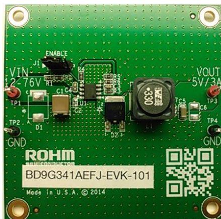
Figure 1. BD9G341AEFJ Evaluation Board
