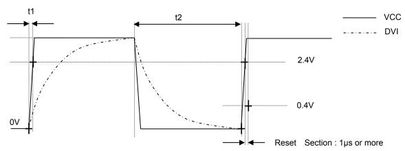
\*Please do the application design to secure Reset section 1µs or more after the reclosing of the power supply.
