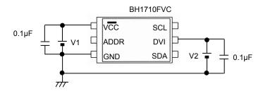
※ Power supply of DVI must stand up later than power supply of VCC stand up, because it is necessary to secure reset section (1µs or more).
