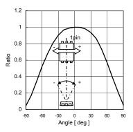
Fig.4 Directional Characteristics 1
