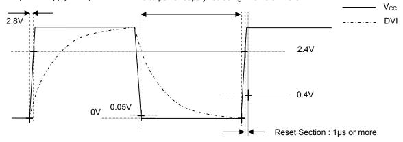
\* Please do the application design to secure Reset section 1µs or more after the reclosing of the power supply.
