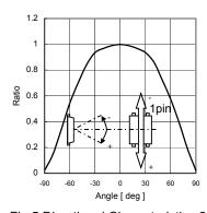
Fig.5 Directional Characteristics 2
