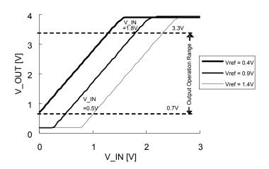
Fig. 5 The relation of V\_IN-V\_OUT at each VREF value (measurement value)
