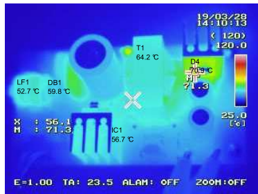
Figure 49. Thermal Image VIN: 90 Vac, IOUT: 4 A
