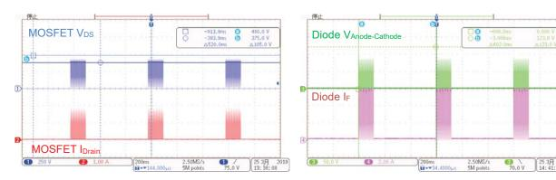
Figure 35. MOSFET V<sub>IN</sub> = 264 Vac, Output Short
