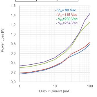
Figure 25. Load Regulation (I<sub>OUT</sub> vs P<sub>LOSS</sub>)
