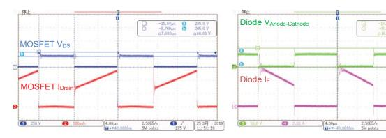
Figure 31. MOSFET  $V_{IN}$  = 90 Vac,  $I_{OUT}$  = 2.0 A
