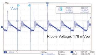
Figure 47. V<sub>IN</sub> = 115 Vac, I<sub>OUT</sub> = 2.0 A
