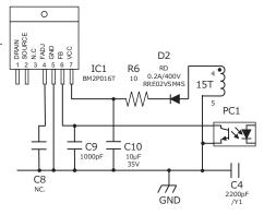
Figure 14. IC peripheral circuit
