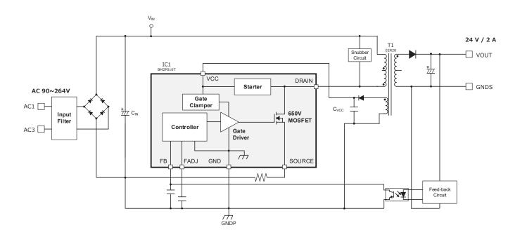
Figure 4. BM2P016T-EVK-004 Application Circuit
