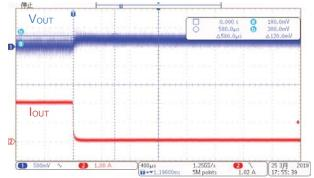
Figure 39. V<sub>IN</sub> = 115 Vac,  $I_{OUT}$  = 10 mA  $\rightarrow$  2.0 A
