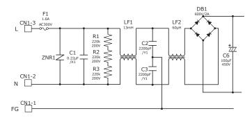
Figure 20. Input filter circuit
