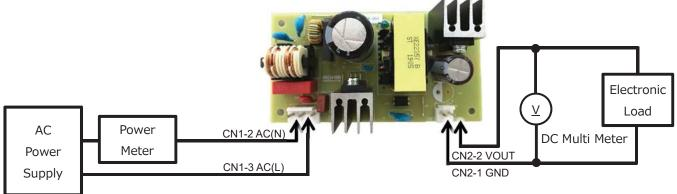
Figure 2. Connection Circuit
