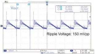
Figure 45. V<sub>IN</sub> = 115 Vac, I<sub>OUT</sub> = 1.5 A
