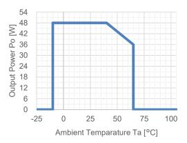
Figure 3. Temperature Deleting curve
