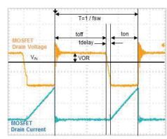
Figure 6. MOSFET Drain Waveform
