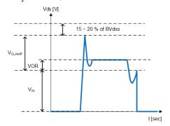
Figure 16. MOSFET Drain Voltage waveform
