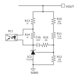
Figure 19. Feed-back circuit
