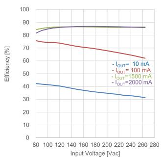
Figure 27. Line Regulation (V<sub>IN</sub> vs Efficiency)
