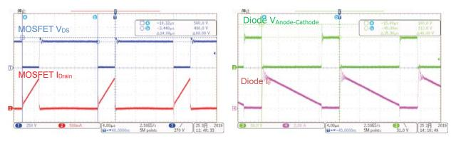
Figure 33. MOSFET V<sub>IN</sub> = 264 Vac, I<sub>OUT</sub> = 2.0 A
