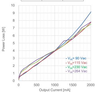
Figure 24. Load Regulation (Iout vs  $P_{LOSS}$ )
