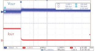
Figure 41.  $V_{IN}$  = 230 Vac,  $I_{OUT}$  = 10 mA  $\rightarrow$  2.0 A
