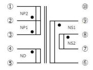
Figure 11. Connection Diagram
