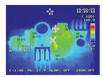
Figure 49. Thermal Image V<sub>IN</sub>: 90 Vac, I<sub>OUT</sub>:1.5 A
