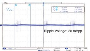
Figure 43.  $V_{IN}$  = 115 Vdc,  $I_{OUT}$  = 10 mA
