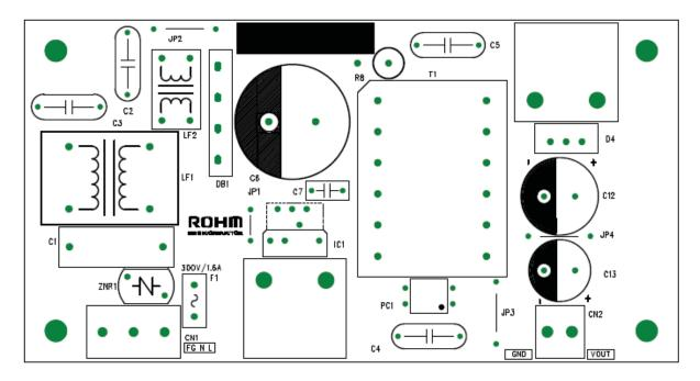
Figure 56. Top Layout (Top view)
