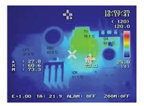
Figure 50. Thermal Image  $V_{IN}$ :264 Vac,  $I_{OUT}$ :1.5 A
