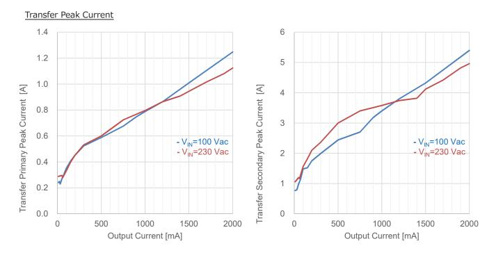
Figure 29. Transfer Primary Peak Current (IOUT vs IPPK) Figure 30. Transfer Secondary Peak Current (IOUT vs ISPK)
