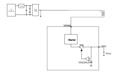
Figure 4. Block diagram of start circuit
