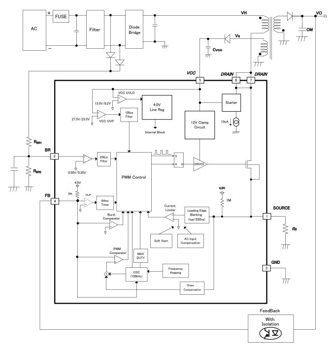
Figure 3. Block Diagram
