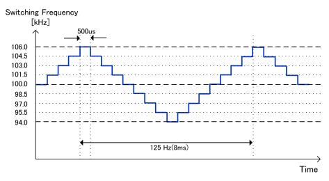
Figure 10. Frequency hopping function
