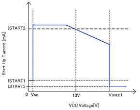
Figure 5. Start current vs VCC voltage
