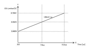
Figure 14. Over current limiter voltage
