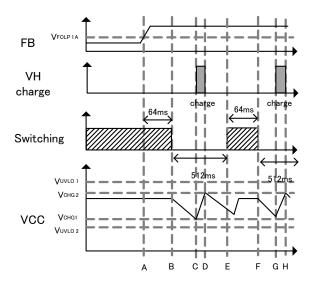
Figure 15. Over load protection (Auto recovery)
