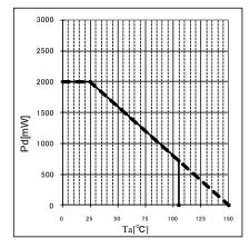
Figure 18. DIP7K Thermal Abatement Characteristics
