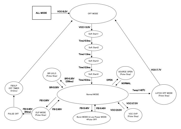
Figure 17. The sequence diagram
