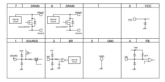
Figure 2. I/O Equivalent Circuit Diagram
