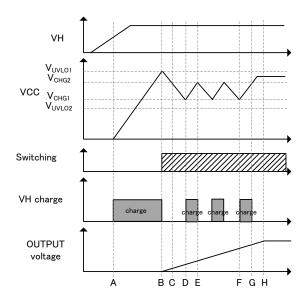
Figure 9. Charge operation VCC pin charge operation
