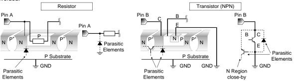
Figure 19. Example of monolithic IC structure
