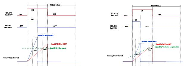
Figure 12. No AC voltage compensation function
