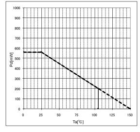
Figure 17. SOP8 Thermal Abatement Characteristics
