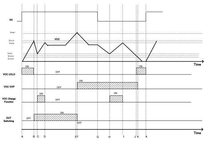
Figure 8. VCC UVLO / OVP Timing Chart
