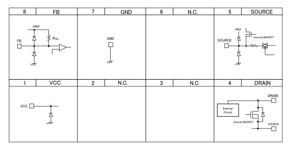
Figure 2. I/O Equivalent Circuit Diagram
