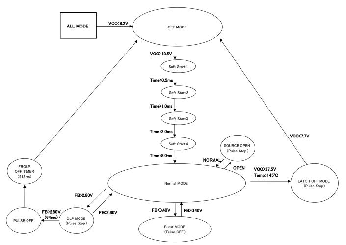
Figure 16. The sequence diagram
