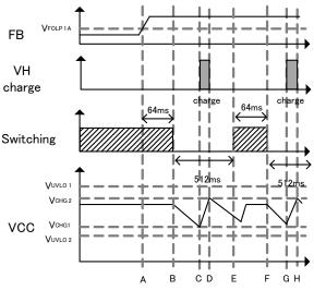
Figure 15. Over load protection (Auto recovery)
