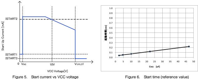
Figure 5. Start current vs VCC voltage
