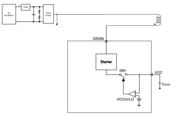
Figure4. Block diagram of start circuit
