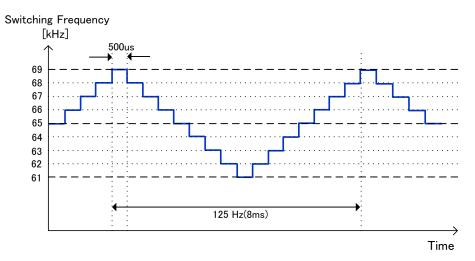
Figure 10. Frequency hopping function
